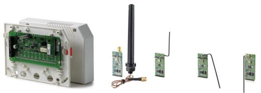
SiWay wireless expander and modules for panels and keypads
