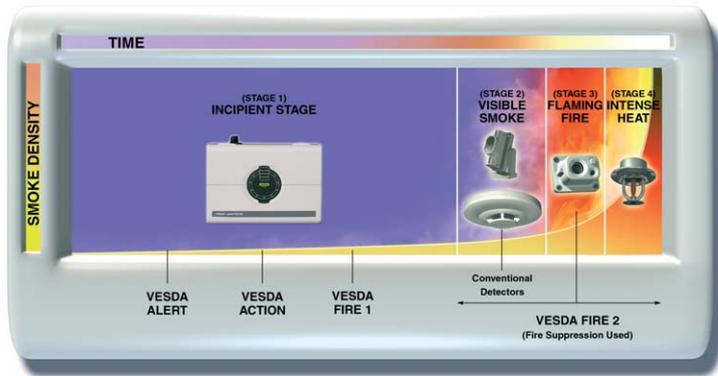
VESDA uniquely monitors the entire progression of a fire — easily detecting smoke long before it is visible and long before any other form of smoke detection.
